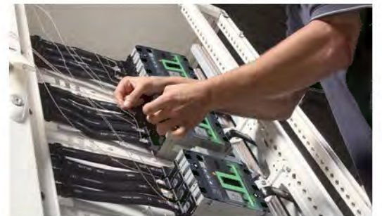
Temperature rise test in laboratory.
